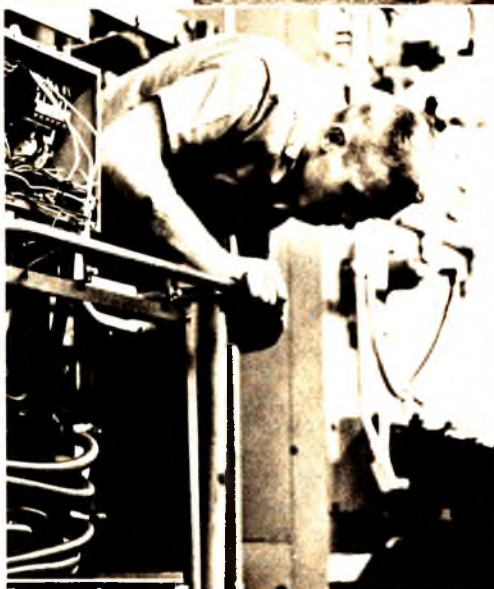
ABOVE: In printing the Sunday school papers, the web of printed paper is split lengthwise by a cutting wheel. The two halves of the roll then separate, passing over diagonally opposite sets of rollers to be repositioned one over the other, ready for the pasting and folcing operations which follow. Adjustment of folding machinery permits a variety of folding and page-size combinations.
