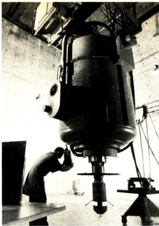
This two-million-volt X ray is used to detect internal voids and inclusions in materials up to 10 inches in thickness with a sensitivity of 1.5 percent.
